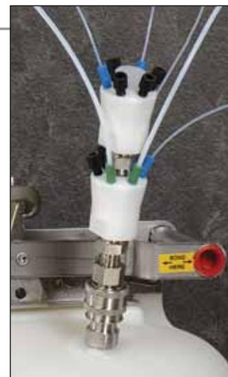
Manifold 86394-27 attached to 86394-31 "stacker"
