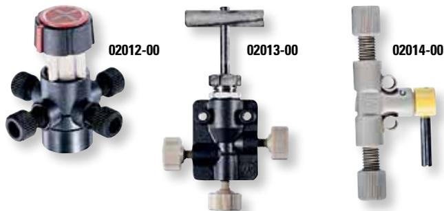
**Switching Valves** offer two flow patterns. Carbon-filled PEEK valve, flangeless Tefzel® ferrules, and Delrin® nuts.
