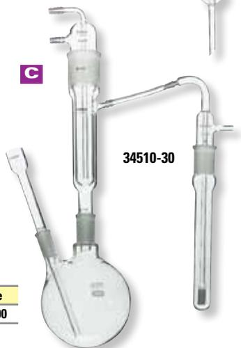
**D Distilling Apparatus for Kjeldahl Determinations** is used to find nitrogen in organic compounds. Perform both digestion and distillation steps in the flask. Includes 200-mm Graham condenser, 500-mL Kjeldahl flask, and connecting tube.
